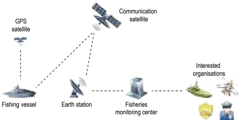
*VMS system: the boat has a VMS unit with an inbuilt Global Positioning System (GPS) receiver and an antenna on board. A satellite picks up the signal and relays it in real time back to earth, where a station collects the data and distributes it to the users.*
